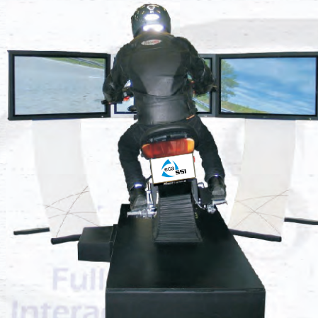
Virtual world graphics integrated with motion base dynamics
